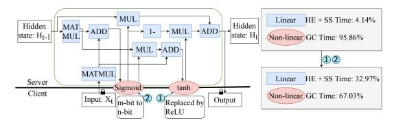
**Fig. 2**. CRYPTOGRU cell with labeled linear and non-linear cryptographic operations. Annotations are referred in Section 3.1, 3.2, and 3.3.
