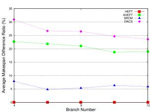
Fig. 7. Average makespan difference ratios under various branch numbers.
