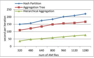
Fig. 11 Time in sec to compute PageRank per iteration with three aggregation approaches with clue-web09 data set on 17 nodes of TEMPEST
