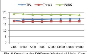
Fig. 8 Speed up for Different Method of Multi-Core Parallelism on 24 cores Compute Node
