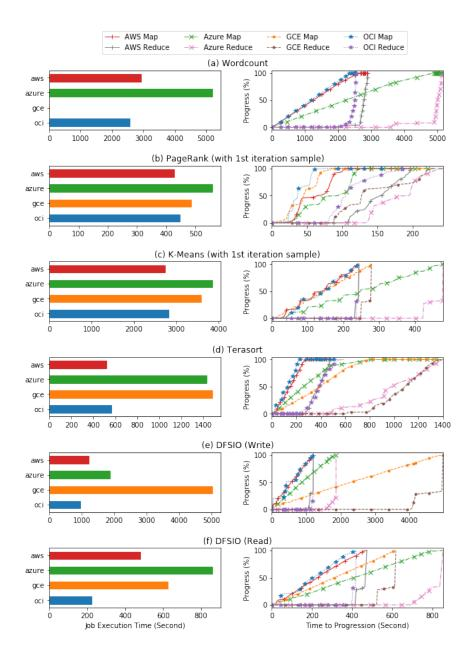
Figure 6.5: Hadoop Workloads on AWS, Azure, GCE and OCI
