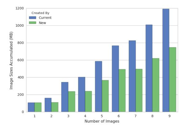
Figure 4.7: Comparison of Container Images for Nginx Version Changes (Current: Built by Official Dockerfiles, New: Built by Common Core Components)
