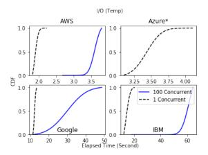
Figure 5.3: Concurrency Overhead with File I/O Intensive Function
