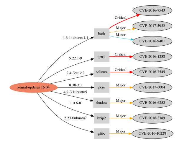
Figure 4.10: Example of Security Vulnerabilities for Ubuntu 16.04 based on Libraries
