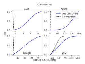
Figure 5.2: Concurrency Overhead with CPU Intensive Function
