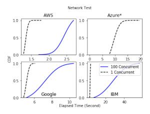
Figure 5.4: Concurrency Overhead with Downloading Objects Function
