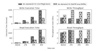
Figure 6.4: TestDFSIO between Block Storage and local NVMe
