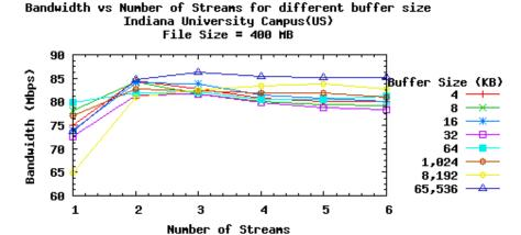
Figure 6: Bandwidth for different buffer size with a fixed file size. (IU-IU settings)
