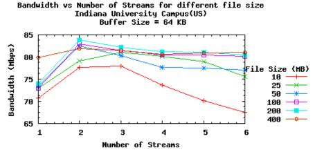
Figure 4: Bandwidth for different file size with a fixed buffer size. (IU-IU settings)
