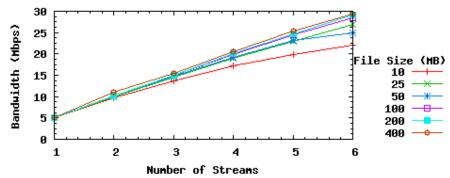
Figure 7: Bandwidth for different file size with a fixed buffer size. (IU-UCSD settings)
