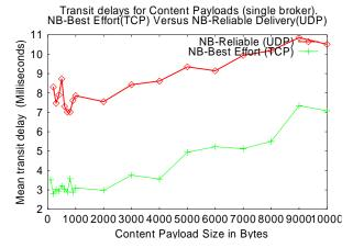
Figure 6: Transit Delay comparison (single broker)
