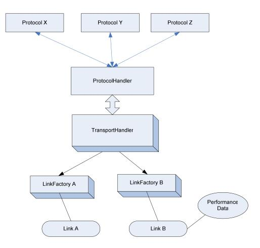
Figure 4 : Transport Framework: Main Components.
