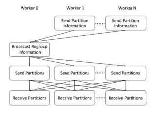
Fig. 5. The Process of Regrouping Array Tables
