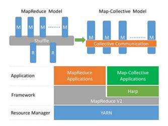
Fig. 2. Parallelism and Architecture of Harp
