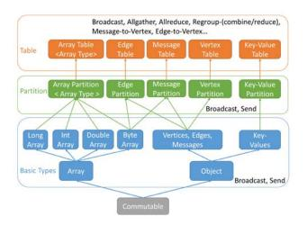
Fig. 3. Hierarchical Data Abstraction and Collective Communication Operations
