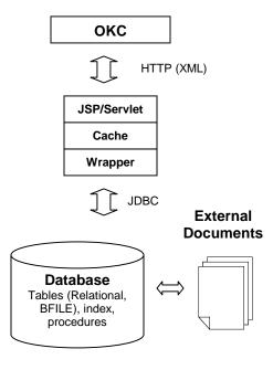
Figure 4. The architecture of the improved hybrid search
