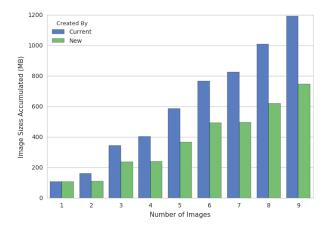
Fig. 7: Comparison of Container Images for Nginx Version Changes (Current: Built by Official Dockerfiles, New: Built by Common Core Components)
