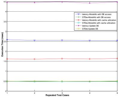
**Figure 10:** Latency and STDev Values for Update DE and More Info Standard Operation (with DB and Memory Utilization)
