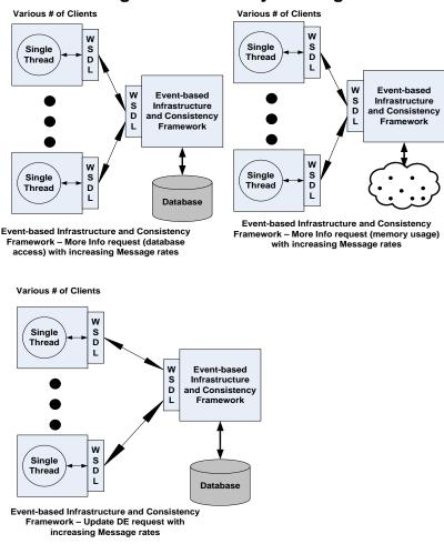
Figure 11: Testing Cases of Scalability Experiment for More Info and Update DE Requests
