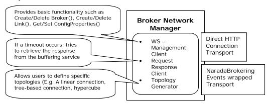
**Figure 4:** Broker Network Manager (aids in deployment of Broker network)
