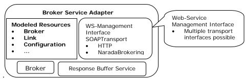
Figure 3: Broker Service Adapter Architecture manages NaradaBrokering brokers
