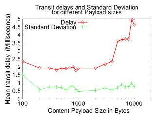
Figure 2: Average delays and standard deviation for message samples
