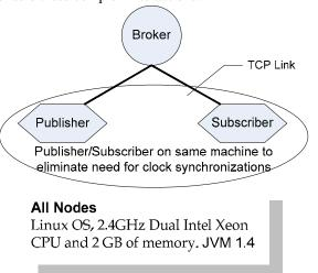
Figure 1: Experimental setup for measuring communication latencies
