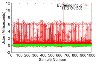
Figure 16: Jitter values comparing Buffering Service Input and TDS Output (Trans-Atlantic)
