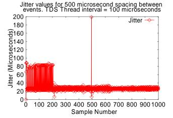
Figure 20: Jitter values for spacing messages with a fixed 500 microsecond spacing between them
