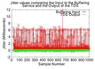
Figure 16: Jitter values comparing Buffering Service Input and TDS Output (Trans-Atlantic)
