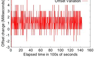
Figure 12: Change of Offset with Time (UK machine no NTP daemon)
