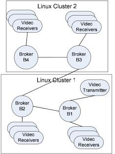
Figure 6: Experimental Setup for Multi-broker measurements
