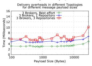
Figure 2: Reliable Delivery Overheads
