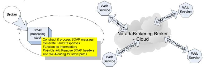
Figure 7: Web Services interacting with the substrate
