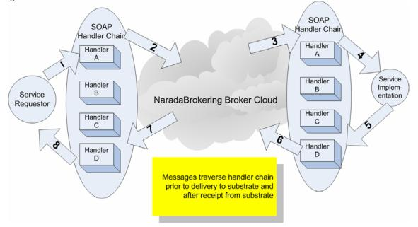
Figure 8: SOAP handler chains and the substrate
