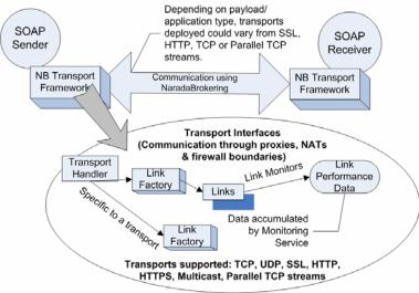
Figure 6: Incorporating support for SOAP in the transport layer
