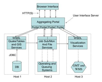
Figure 1 The SERVOGrid architecture consists of distributed Web Services accessed through the QuakeSim user portal. Solid arrows represent network connections (SOAP over HTTP unless otherwise indicated). Broken arrows represent interactions with the local operating system. As shown in the figure, the portal may serve (in effect) as the state and workflow management system for the services. We also provide these as separate services through the HPSearch and WS-Context development work.
