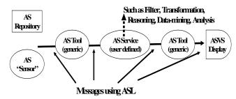
Figure 2: Application Specific Information System architecture for application specific Sensor Filter Grids.
