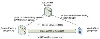
Fig. 9. Scenario for WS-Addressing example
