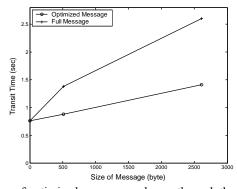
**Fig. 11.** Round trip time of optimized message exchange through the HHFR high performance channel compared with full message exchange
