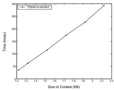
Fig. 12. Time to finish Context-store request message processing (i.e., T<sub>time-in-axis</sub>)
