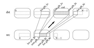
Fig. 10. Illustration of sendLoop operation for remap
