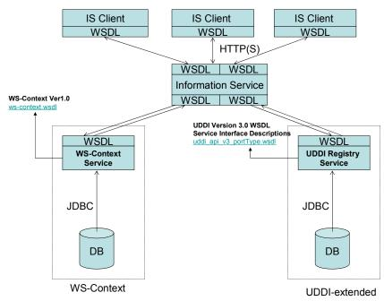
Figure 3: Architectural Design of an Information Service
