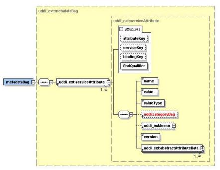
Figure 1: XML Schema for service metadata
