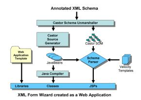
Fig. 2. The XML Schema Wizard simultaneously generates user interfaces, in-memory data bindings, and actions links between interface elements and data objects for an XML schema.
