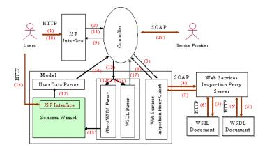
Fig. 3. A usage scenario illustrates the interaction of WSDI and Schema Wizard components.
