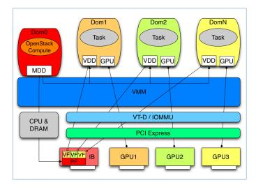
Fig. 3. PCI Passthrough and SR-IOV for InfiniBand and GPUs
