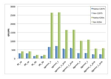
Fig. 4. GPU Fast Fourier Transform & Matrix Multiplication performance
