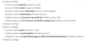
Figure 4. An example index configuration file.
