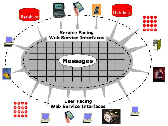
*Fig. 2: A Peer-to-Peer Grid constructed from Web Services with both userfacing and service-facing ports to send and receive messages*
