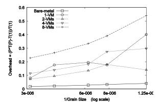
Figure 14. Total overhead of the Kmeans clustering – overhead against the 1/ grain size, grain size = number of 2D data points per parallel task (Number of MPI Processes = 128)
