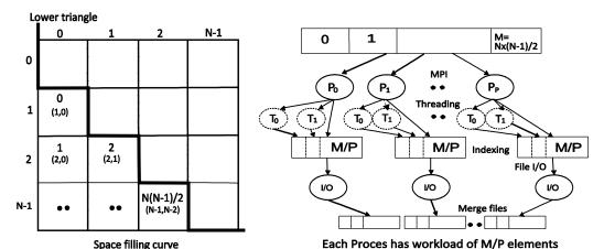
Figure 4. Task decomposition (left) and the MPI (right) implementation of SW-G pairwise distance calculation application.
