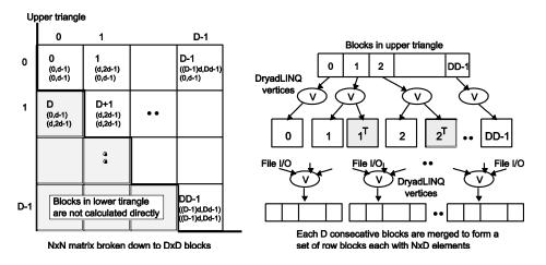
Figure 3. Task decomposition (left) and the DryadLINQ vertex hierarchy (right) of the DryadLINQ implementation of SW-G pairwise distance calculation application.
