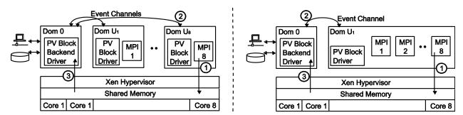
Figure 18. Communication between dom0 and domU when 1-VM per node is deployed (left). Communication between dom0 and domUs when 8-VMs per node were deployed (right).
