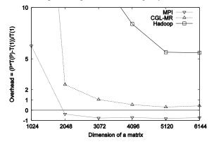
Figure 8. Overhead induced by different parallel programming runtimes for the matrix multiplication application – overhead against the dimension of an input matrix.
