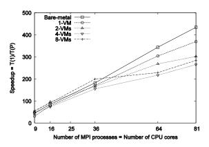
Figure 11. Speed-up of the matrix multiplication application – Speedup against the number of MPI processes = number of CPU cores used (Fixed matrix size = 5184x5184).
