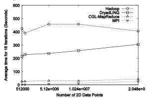
Figure 7. Overhead induced by different parallel programming runtimes for the Kmeans Clustering application – overhead against the number of 2D data points clustered (Note: Both axes are in log scale)
