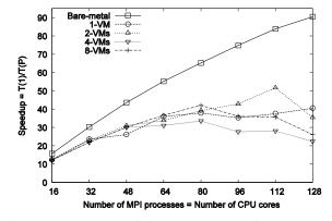
Figure 13. Speed-up of the Kmeans clustering – speedup against the number of MPI processes = number of CPU cores used (Number of data points = 860160)
