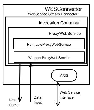
Figure 3. WS Proxy Architecture
