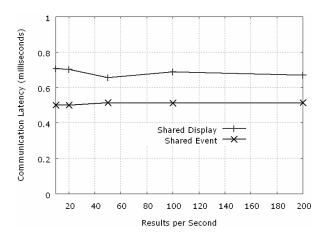
Figure 6. Network Overhead for Collaborative Interactions under Varying Results Stream Rates
