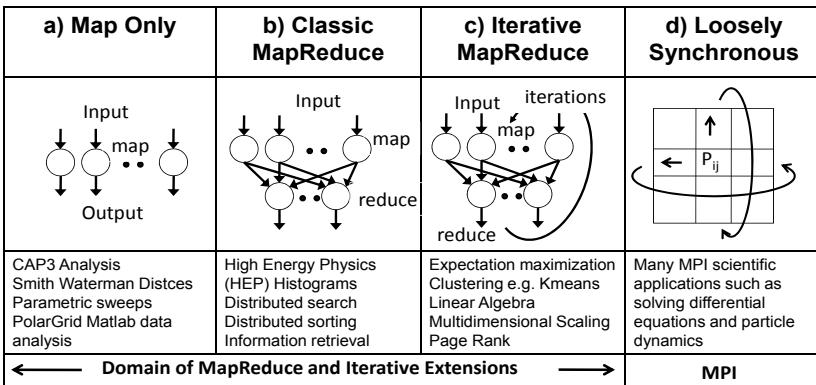
Fig 1: Four applications classes and their mapping to run time/ programming models
