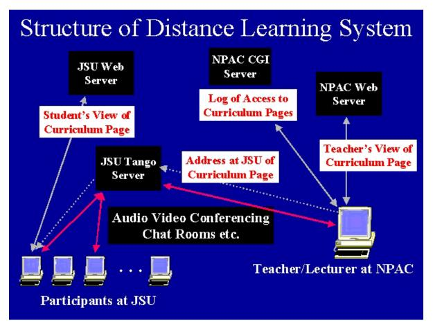
Figure 9: Dual-server Network Architecture
