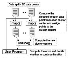
Figure 5. MapReduce for Kmeans clustering
