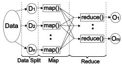
Figure 1. The MapReduce programming model
