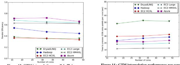
Figure 13: GTM interpolation parallel efficiency
