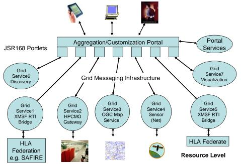
Figure 3: Grid Enhanced XMSF based Modeling and Simulation System with Clients, Portal, Grid Services and Resources including HLA/DIS subsystems
