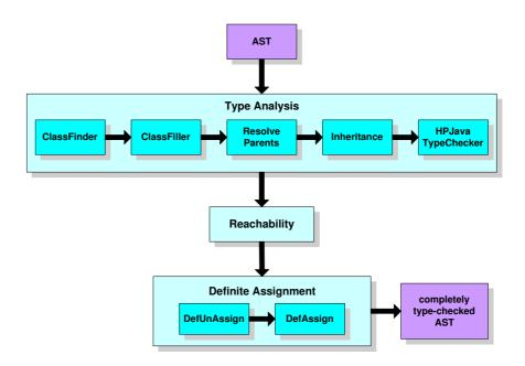
Figure 5. The Architecture of HPJava Front-End.
