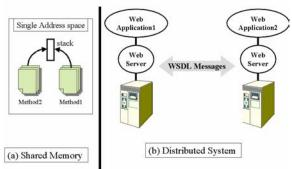
Fig. 7. Schematic of two bindings of a Web Service (a) Single address Space and (b) Distributed
