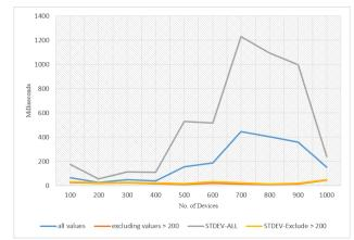
Figure 12 Latency with varying number of devices – Kafka. The average latency and standard deviation is shown. Also averages calculated with ommitting values over 200 are shown.
