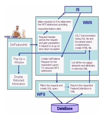
Figure 8 : getFeatureInfo work flow.
