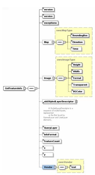
Figure 2 : GetFeatureInfo Request Schema.
