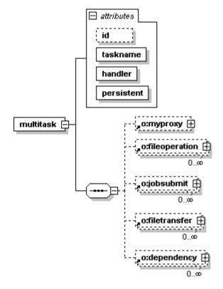
Figure 2 XML schema of multitask represents a DAG. It shows the relationship of Grid tags by defining dependency tag in GTLAB.
