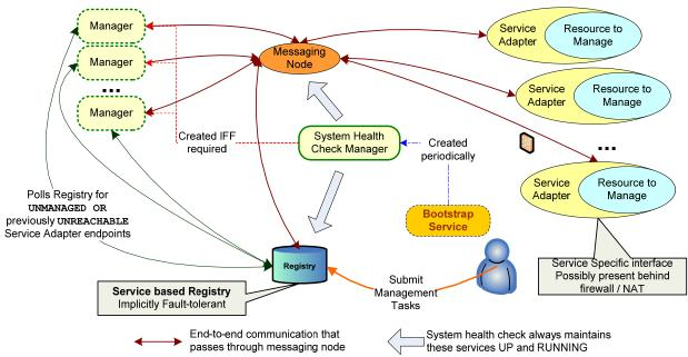
Figure 1 Overview showing components of the Management Architecture
