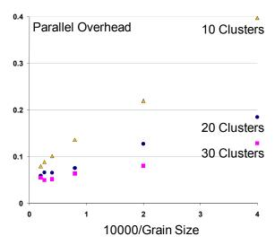
Figure 2. Parallel Overhead for GIS 2D DA Clustering on Intel 8b using C# with 8 threads (cores) and CCR synchronization. We show 3 values (10.20,30) for the number of clusters and plot against the reciprocal of the number of data points per thread
