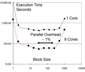
Figure 4. Timing of 4096X4096 Parallel Matrix Multiplication as a function of block size for 1 and 8 cores on Intel8b
