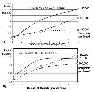
Figure 5. Scaled Run time on Intel8b using Vista and C# with CCR for synchronization on Clustering Kernel for three dataset sizes with 10,000 50,000 or 500,000 points per thread(core). Each measurement involved averaging over at least 1000 computations separated by synchronization whose cost is not included in results (see text)
