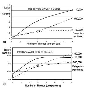
Figure 5. Scaled Run time on Intel8b using Vista and C# with CCR for synchronization on Clustering Kernel for three dataset sizes with 10,000 50,000 or 500,000 points per thread(core). Each measurement involved averaging over at least 1000 computations separated by synchronization whose cost is not included in results (see text)
