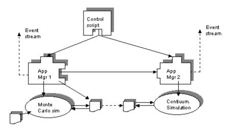
Figure 5. Two coupled Chemical Engineering simulation programs. Application Manger 1 signals Application Manger 2 when the Monte Carlo simulation completes a time step and the associated output state files have been migrated. Upon receipt of the message Application Manager 2 runs the continuum simulation. When this terminates control is returned to the first AM.
