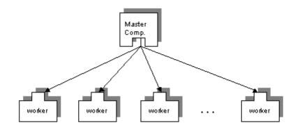
Figure 6. Two types of components, master and worker are used to partition the problem and distribute the work
