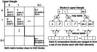
Figure 3. Twister implementation of the SW-G distance calculation program.
