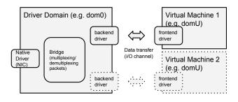
Figure 1: Xen Networking with Paravirtualized Network Devices
