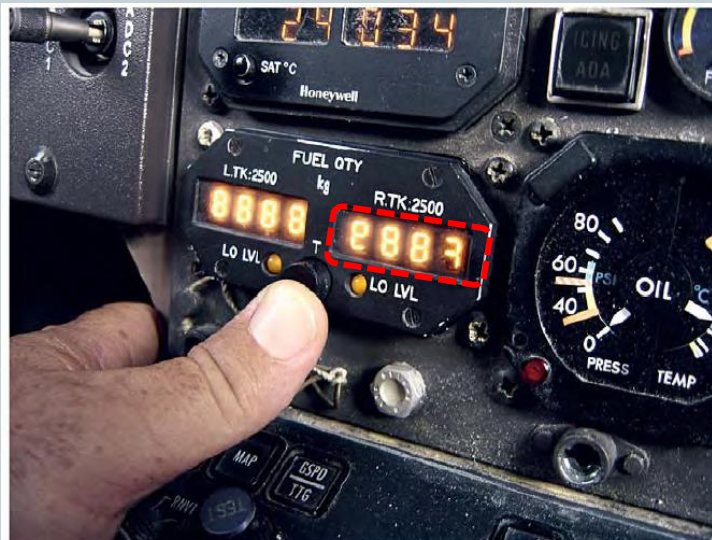
Photo 1: The FQI installed on TS-LBB before replacement.
