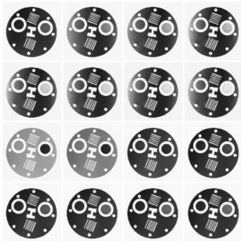
Figure 2.6. Series of Images of an Imaging “Phantom”: The phantom contains regions with different T1 and T2 relaxation times. Adjusting imaging parameters changes the contrast between the regions.
