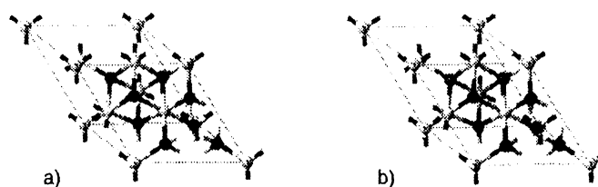
FIG. 1. Primitive cell of: (a) c\text{-Si}_3\text{N}_4 ; and (b) c\text{-Si}_5\text{AlON}_7 (model B2). Dark (light) balls are N (Si) atoms. In (b) the gray ball is the substituted O and the central ball is the substituted Al.
