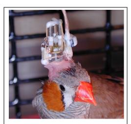
**Fig. 2** – Motorized microdrive implanted on a zebra finch.
