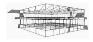
Figure 3: (left) Input interface to the CMA model in the WBCSim PSE [43]. (right) Wireframe model of a wood-based composite showing failed layers (gray) and active layers (black), and the orientation of fibers in each layer. In this figure, the second layer has failed.
