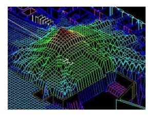
Figure 6: (left) Example outdoor environment for designing a wireless communications system in the S<sup>4</sup>W PSE [51]. (right) Propagation coverage prediction around the region of interest in the environment.
