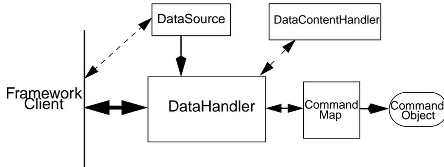
This diagram shows the major elements comprising the JAF architecture. Note that the framework shown here is not bound to a particular application.
