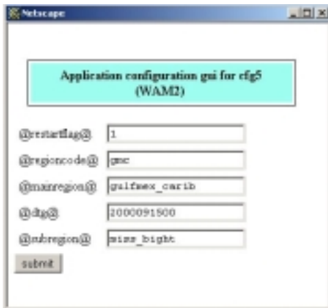
Figure 4: Automatically generated GUI for the WAM model by applying XSL transformation to the application descriptor which defines five input parameters: restartflag, regioncode, mainregion, dtg and subregion
